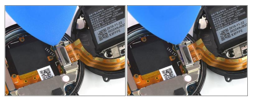
(i) The metal shield is held in place by a clip.
