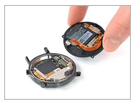
• Separate the back cover assembly from the watch case.
