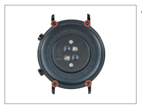
Use a T2 Torx screwdriver to remove the four 3.6 mm screws securing the back cover assembly.
