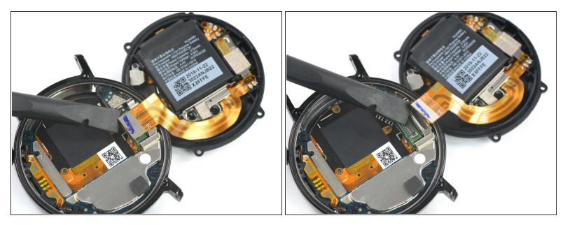
• Use a spudger to disconnect the back cover assembly.
