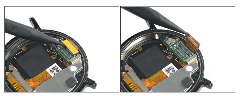
• Use the pointed end of a spudger to disconnect the display flex cable from the motherboard.
