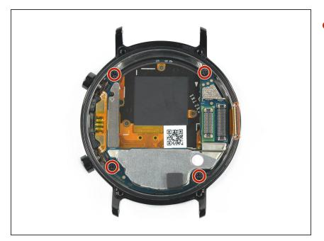
Use a Phillips #00 screwdriver to remove the four 2.3 mm screws securing the motherboard.
