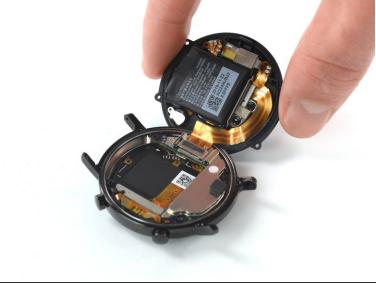
Carefully swing the back cover assembly open to an upward position.
