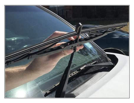
Pull towards the shaft of the windshield wiper, removing it from the clip.
