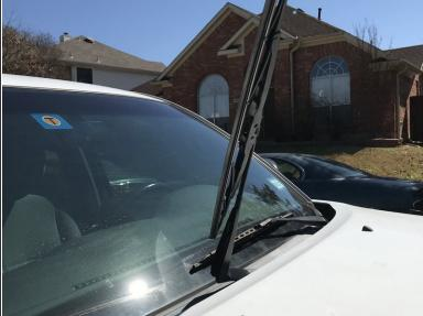
Turn the wiper so that it is tangent to the wiper shaft.
