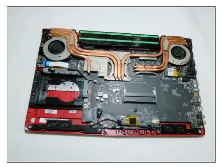
Reorient the computer, if necessary, with a 180 degree turn so that the speakers face you.
