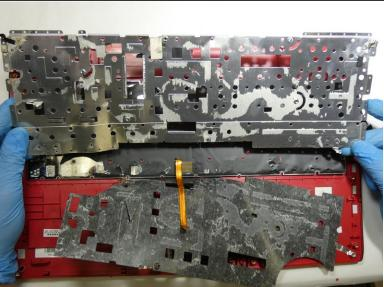
Using a metal spudger, pry the keyboard metal backing away.
