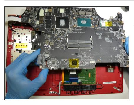
Gently lift away the motherboard, directly upward.
