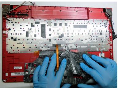
Peel back the adhesive black lining attached to the keyboard.
