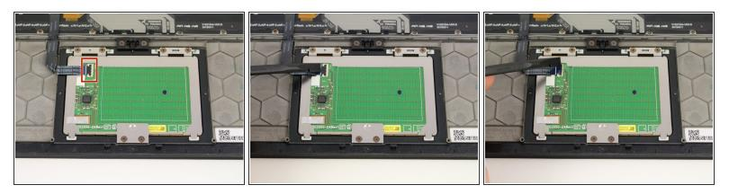
• Use a spudger to lift the hinged black tab of the <u>ZIF connector</u> on the trackpad.
