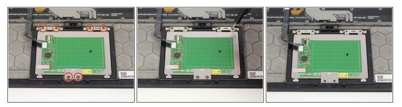
Remove the six 2.2 mm screws from the trackpad with a Phillips #00 screwdriver.
