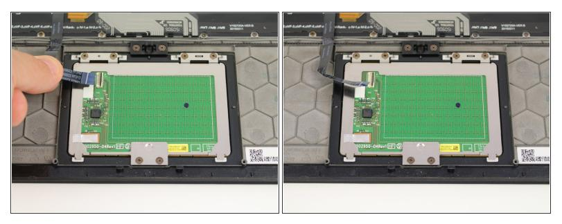
• Pull the cable out from the connector with your fingers.
