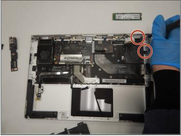
• Remove the four screws attached to both fans, and the back connector strip (the long metal piece furthest from you with screws in it) with a Phillips #0 screwdriver.
