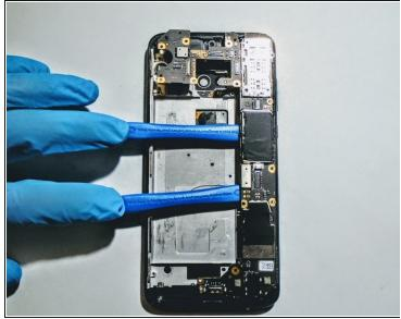
Insert the plastic opening tool under the right and top of the motherboard, and pry it free from the body. To reassemble your device, follow these instructions in reverse order.
