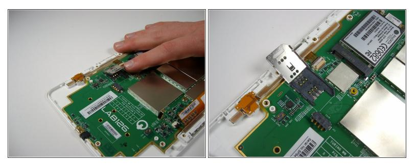
• Lift the now unlocked case up on its hinges to reveal the SIM card slot.
