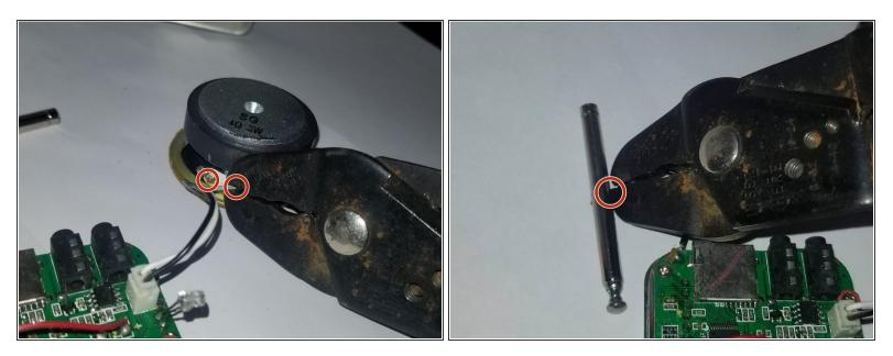
• Cut the wires of the **Speaker** and the **Antenna** as close to the old parts as possible.
