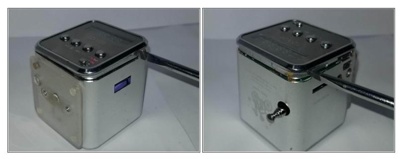
• Use a plastic opening tool to remove the face of the radio.
