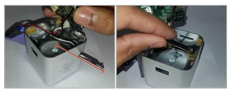
Place the face of the radio to the side with the battery and thread the Antenna through the inside compartment to remove it.
