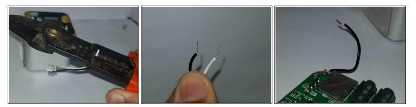
• Strip the ends of the wires where you cut so that some wire is exposed to solder to the new parts.
