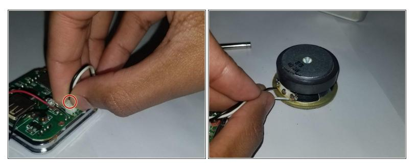
• Unplug the **Speaker Wire** from the circuit by pinching the small clip and wiggling it out.
