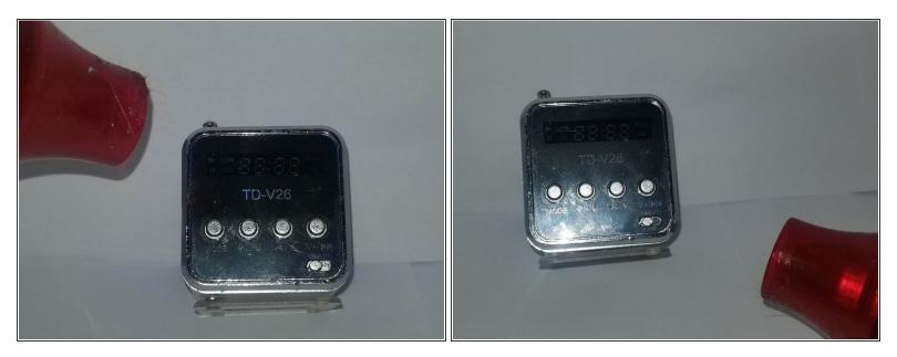
• Using a heat gun, loosen the glue holding the face of the radio.
