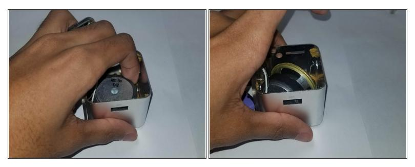
• Pry out the **Speaker** from its holding position in the frame of the radio.
