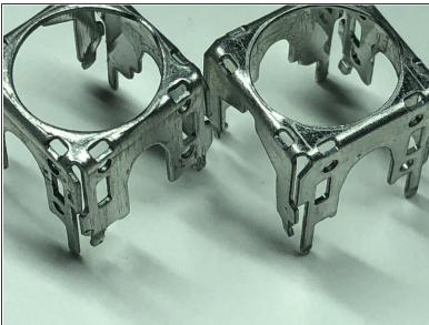
Last we have the bodies. These are both stamped out of the same thickness material, but the older revisions appear to have slightly more metal near all corners allowing tighter gaps. This may allow more dust and debris to get into the newer revision switches.
