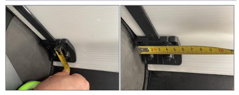
• Select the right replacement by measuring the diameter and width of the wheel.
