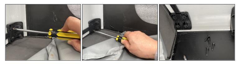
• Remove the screws securing the wheel clip inside the case.
