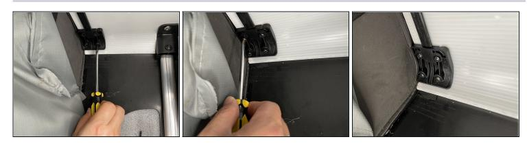
• Tighten the screws that hold the clip back in place.
