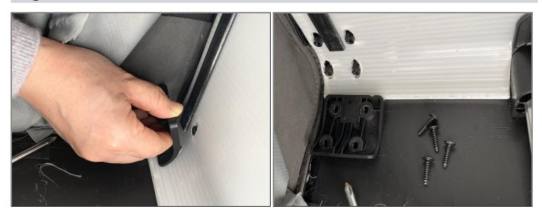
• Pull out the clip securing the wheel to the case.
