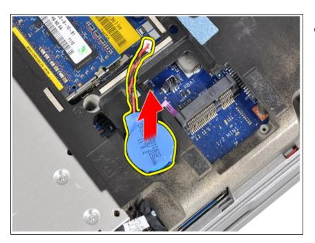
Remove the coin-cell battery from the computer.
