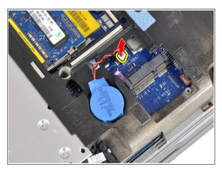
Disconnect the coin-cell battery cable from the system board.
