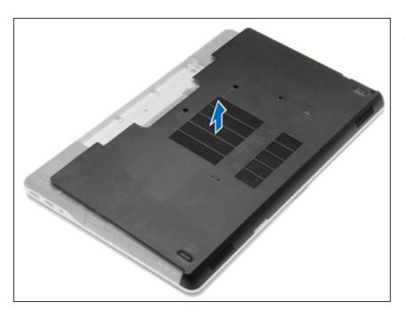
Lift the base cover and remove it from the computer.
