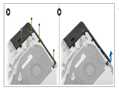
Remove the screws that secure the right base corner cap, lift and remove it from the computer.
