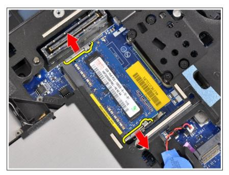
Pry the securing clips away from the memory module until it pops up.
