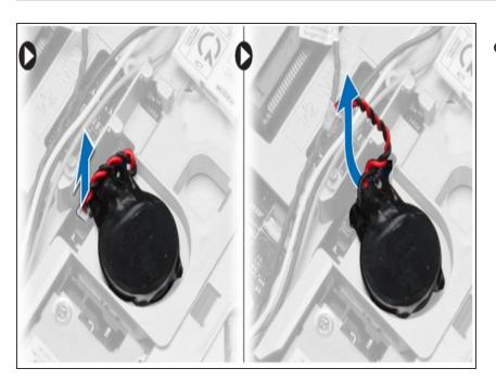
Disconnect the coin-cell battery cable, and take out the coin-cell battery pointing up.
