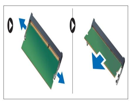
Open up the clips away from the memory chip until it pops up out of its slot. Take out the memory clip from the system board's connector.
