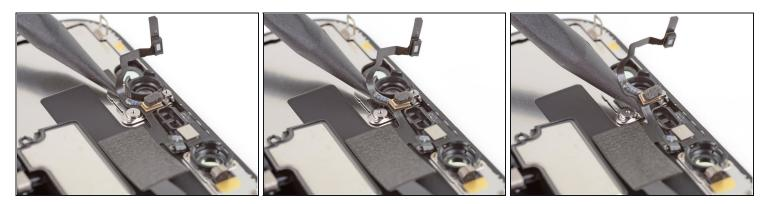
• Use the point of a spudger to lift and separate the microphone from its notch in the front panel.
