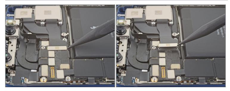
• Use a spudger or a fingernail to disconnect the first camera cable connector by prying it straight up from its socket.
