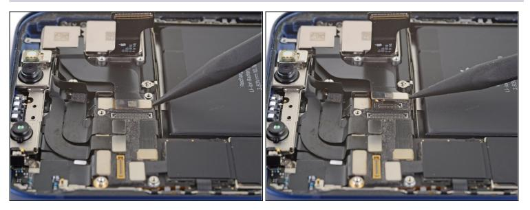
• Use a spudger or a fingernail to disconnect the second camera cable connector by prying it straight up from its socket.
