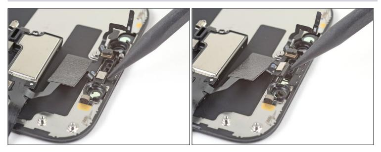
• Use the point of a spudger to lift the proximity sensor and flood illuminator module out of its notch in the front panel.
