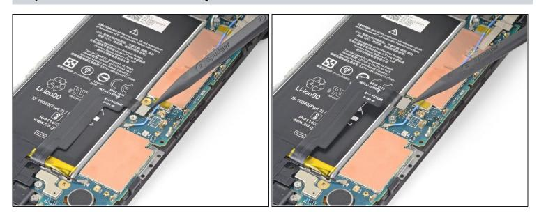
• Use the tip of a spudger to disconnect the battery cable from the motherboard.
