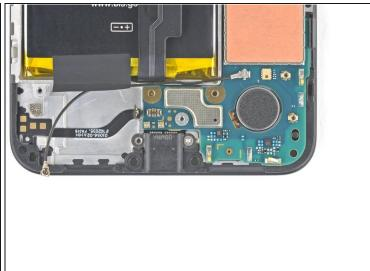
Use a T3 Torx screwdriver to remove the 2.1 mm-long screw securing the charging port.
