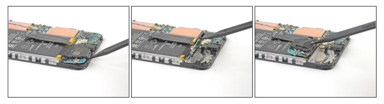
Insert the tip of a spudger underneath the loudspeaker assembly.
