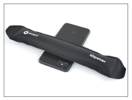
Use an iOpener or heat gun to apply heat for one minute to the outside of the back cover around the fingerprint sensor to soften the adhesive.
