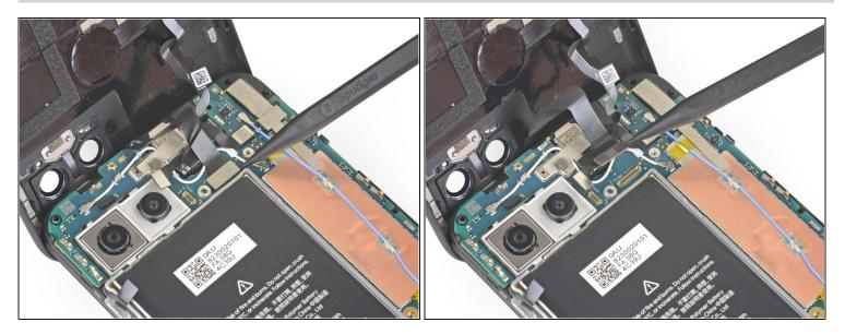
• Use the tip of a spudger to pry up and disconnect the front sensor array cable.
