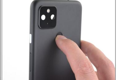
• Use your finger to push the fingerprint sensor through the back cover until it begins to separate.
