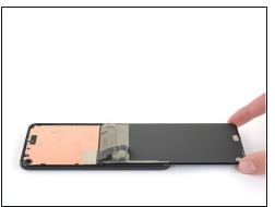
• Lift from the top edge and swing the screen over the bottom edge until you can rest it glassside down.
