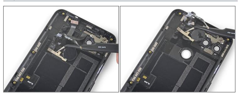
Remove the fingerprint sensor.
