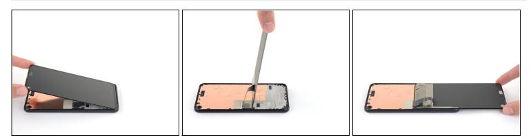
• Lift from the top edge and swing the screen over the bottom edge until you can rest it glassside down.
