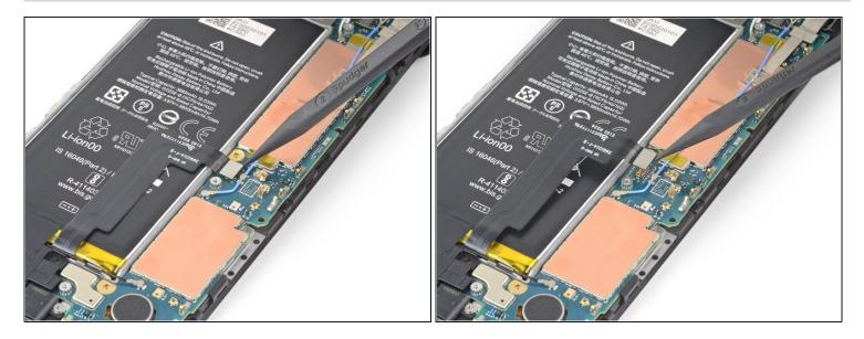
• Use the tip of a spudger to disconnect the battery cable from the motherboard.
