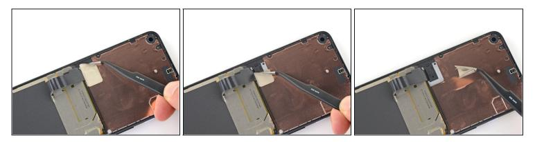
• Use your fingernail or a pair of tweezers to carefully peel off the tape covering the screen connector.
