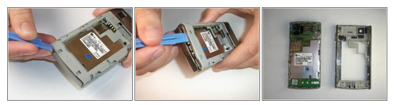
• Flip your phone over to the battery side. Locate the seam near the bottom of the phone between the plastic case and the metallic case. Like the previous step, wedge the opening tool into the seem, and slide it across. Then, pry the two pieces apart. Your phone should now be in two pieces.
