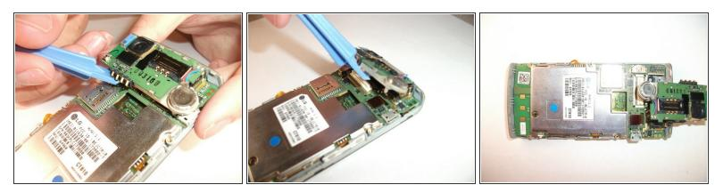
To get access to the third tab, insert your plastic opening tool underneath the speak/camera panel, and gently pry at it. Do not fully remove the board though! It should still be attached to the motherboard by a red and black wire. Images two and three show the tab is red.
