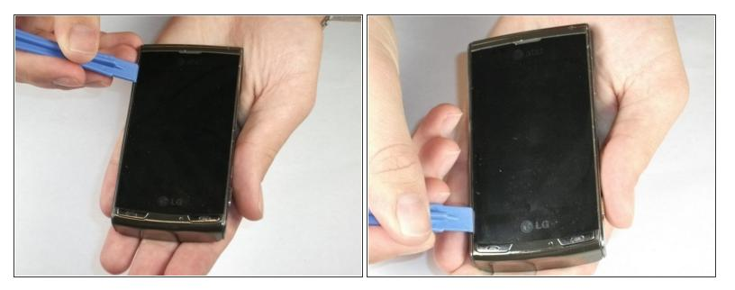
• With the screws set aside, wedge your plastic opening tool in between the screen and the case surrounding it. Gently move the tool along the edge to loosen the screen from the casing. Do this again on the other side as well. The screen and case won't be completely separate in this step.
