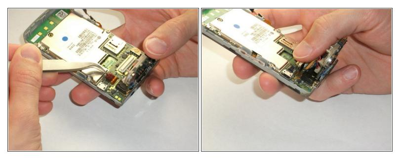
• To loosen this tab, use your metal tweezers to lift the side of the tab shown in image 1. You only need to gently lift it, it should pop off quite easily.
