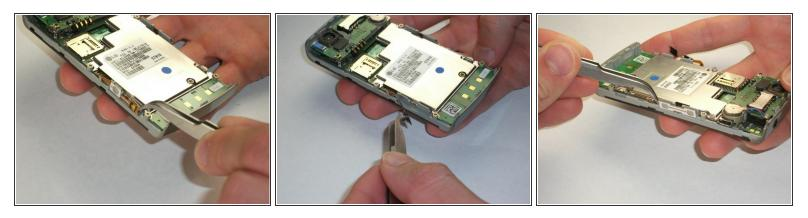
• The first two tabs are the easiest to remove. Take your metal tweezers and gently separate the white panel from the gray surface they are attached to. Do the same thing to the white panel on the other side of the phone (as shown in image 3).
