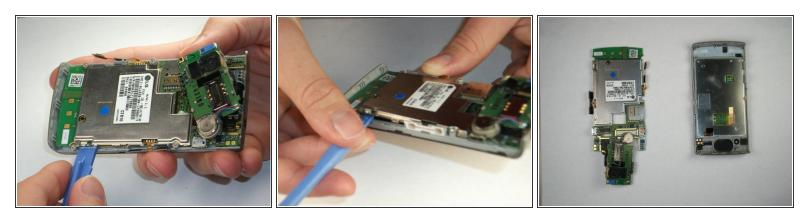
• With all three tabs removed, its time to separate the motherboard from the other casing! Insert the plastic opening tool as shown, and gently pry the motherboard from its case. Make sure to do this on all sides before fully prying the two apart. The third image shows the motherboard on the left, and the second casing on the right.
