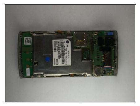
Here is a top-down view of what your phone should look like. There are three yellow tabs that need to be loosened in order to remove the motherboard. The third tab is located underneath the speak/camera board in red.
