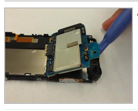
To remove the motherboard, apply upwards pressure on the bottom green tab.
