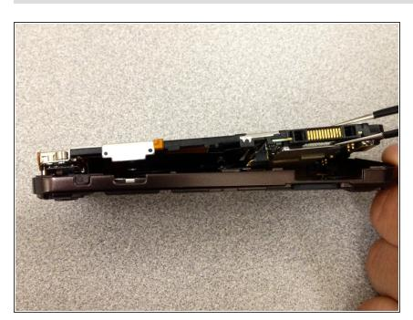
Now that the faceplate is off, use tweezers to separate the backplate from the inner manifold.
