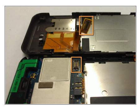
With both insides of the phone exposed, gently detach the ribbon cable connecting the two inner sides. You can now separate the two sides of the phone.
