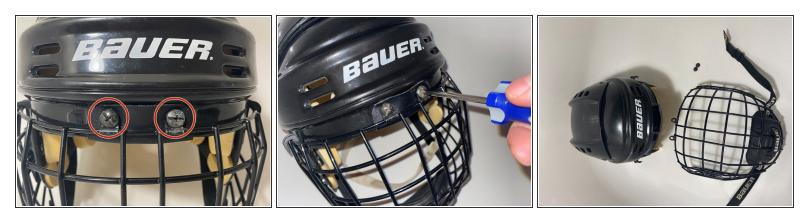
• Unscrew the hinge clips from the front of the helmet.
