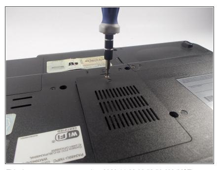
Screw the back plate of the RAM back onto the device.
