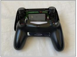
Detach the back shell from the rest of the body by pulling the front shell and back shell apart simultaneously.
