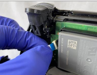
Place the ribbon attached to the back shell on the circuit board and press down so both compartments get attached.
