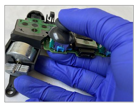
Take the left joystick and put it back on until the click is heard which confirms that the joystick is firmly held on.
