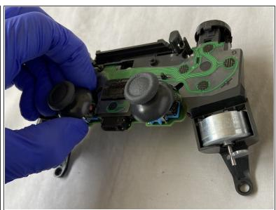
Remove the left joystick by pulling it upwards until it pops off.
