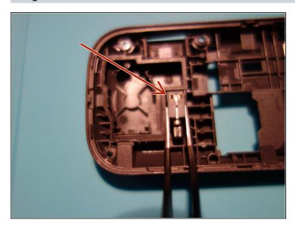
• Remove the vibracall engine with the <u>tweezers</u>
