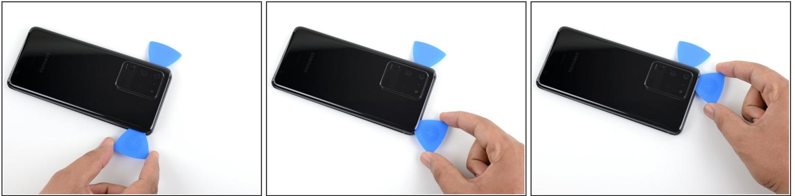
**⚠** The glass near the corners of the back cover is curved and very susceptible to cracking. Be gentle during this step to prevent damaging your back cover.
