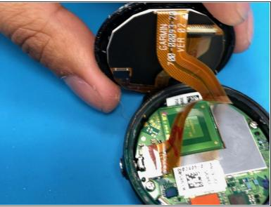
Once opened, remove carefully the screen's ribbon cable. It is recommended to use plastic tools during the whole process. You should consider that the battery is still connected.
