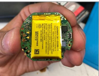
Here you can replace the battery if needed. It is soldered through two cables to the clock's motherboard.
