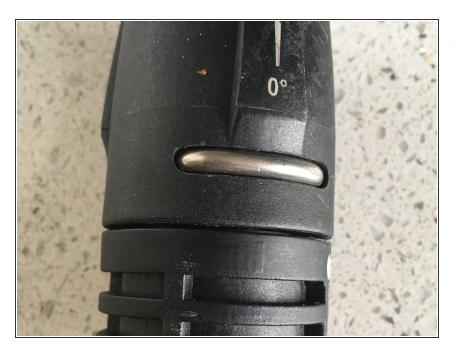
Once this pin has been backed out far enough, remove it with channellock pliers. Careful, all internal parts tend to fall out once this pin has been pulled out.
