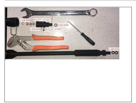
Pictured all labelled parts in exploded view and tools used.
