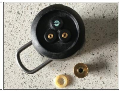
Replace required part and reassemble. Use channellocks to pinch metal pin to fit it back in the holes. To properly remove an o-ring, view the following video. For tough to remove o-rings, also pinch it with a cloth. <a href="https://www.youtube.com/watch?v=EDiDoJCf...">https://www.youtube.com/watch?v=EDiDoJCf...</a>
