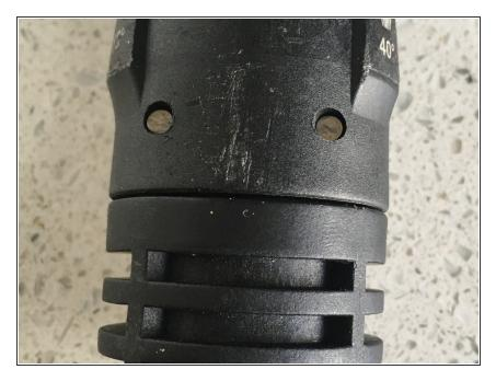
Use punch and hammer to back out metal pins seen here.
