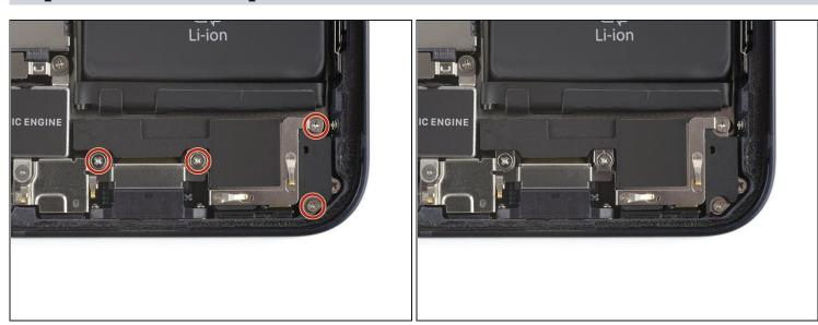
• Remove the four 1.5 mm-long Phillips #000 screws securing the speaker.
