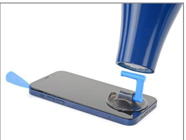
• Use a hair dryer to heat the left edge of the iPhone for 90 seconds or until the screen is slightly too hot to touch.
