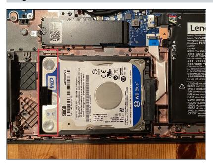
Finally, align the hard drive and push on the marked end.
