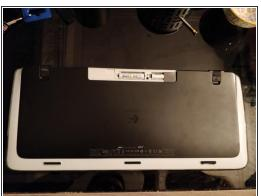
Once the battery location open, replace the original battery with new rechargeable batteries.
