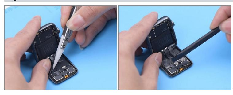
• Peel off the tape covering the display flex cables with tweezers. Please do not damage the flex cables while peeling off. Then disconnect the flex cables.
