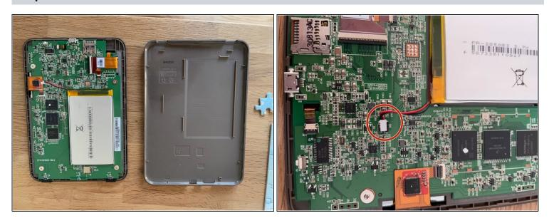
Now disconnect the battery cable. Carefully pry it off from below.
