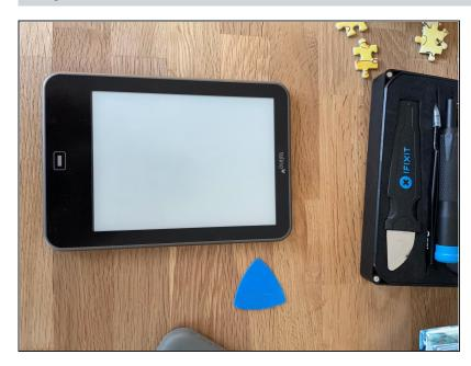
First, open the edge of the Tolino with a spudger or pick. The lid is only clipped and can be opened easily.
