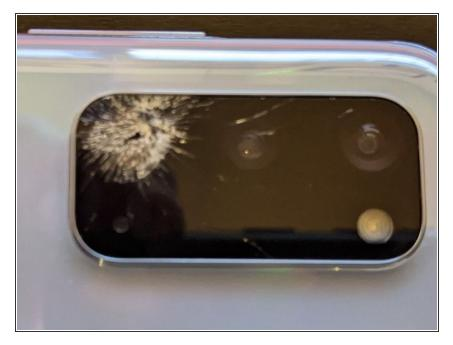
So you broke your glass, step one complete. Note: The lens is held on with adhesive so we will need to heat the area. A blow dryer will work or a heat gun will get the job done. If you have a puncture you can use some tweezers to begin pulling up the glass there. Please NOTE, look at the next step photo to see where the lens resides.
