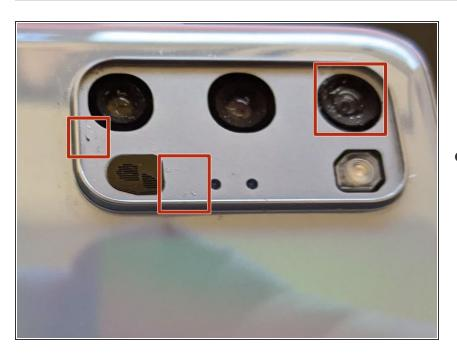
Once you have removed all glass, ensure there is no adhesive left on the silver plate where your new adhesive will go. I used alcohol wipes and my tweezers to ensure the area was adhesive free. Also, ensure there is no glass inside the cameras themselves when cleaning. I used an alcohol wipe to ensure it was clear. Red boxes show leftover glass.
