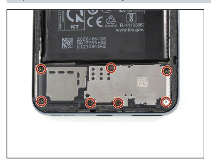
Use a Phillips #00 screwdriver to remove the seven 3.6 mm-long screws.
