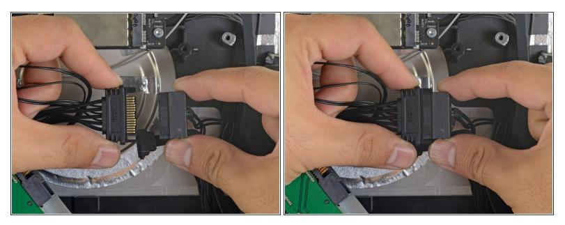
• Connect the iMac's SATA power cable to the other end of the new sensor-enabled SATA cable.
