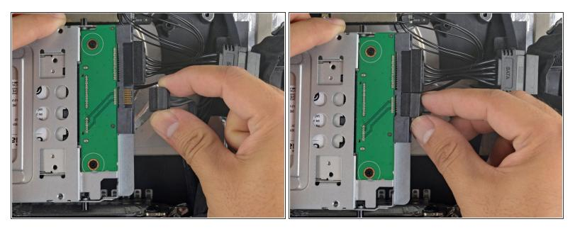
• Connect the iMac's SATA data cable to the enclosure.
