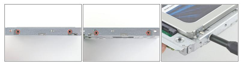
Use a Phillips screwdriver to install the four silver screws (two on each side) along the edges of the SSD to secure it to the enclosure.
