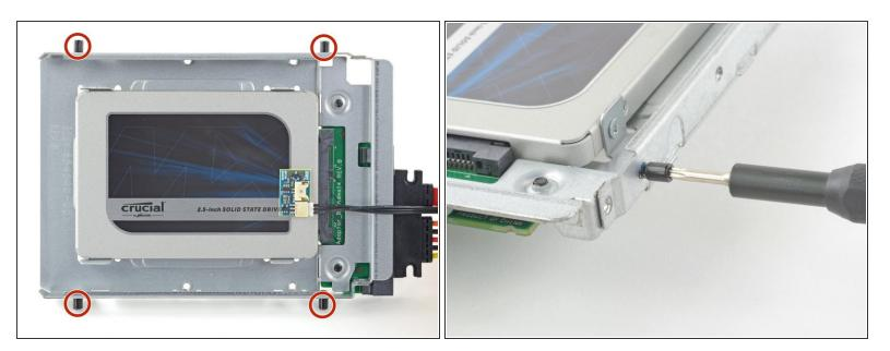
• Use a T8 driver to install the mounting pins from the old hard drive onto the sides of the enclosure.
