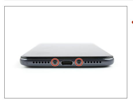
Remove the two 2.7 mm-long Torx T3 screws from the bottom edge of your phone.
