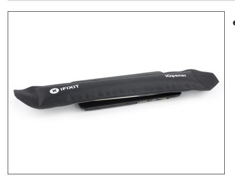
Apply a <u>heated iOpener</u> to the screen to loosen the adhesive underneath. Apply the iOpener for at least two minutes.
