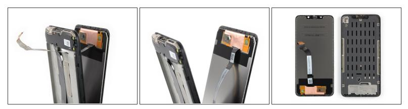
• Thread the display flex cable through the gap in the midframe and remove the display.
