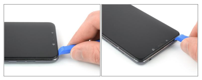
Slide the opening tool along the top edge of the phone to release the plastic clips holding the back cover in place.
