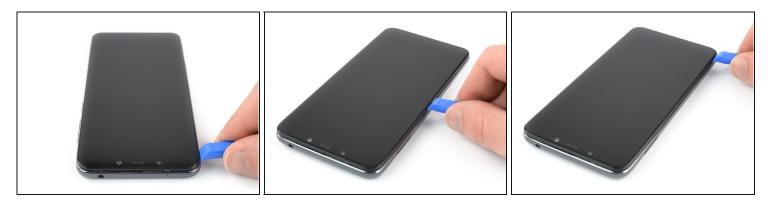
• Slide the opening tool along the left edge of the phone to release the remaining plastic clips.
