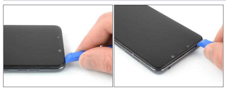
Slide the opening tool along the top edge of the phone to release the plastic clips holding the back cover in place.
