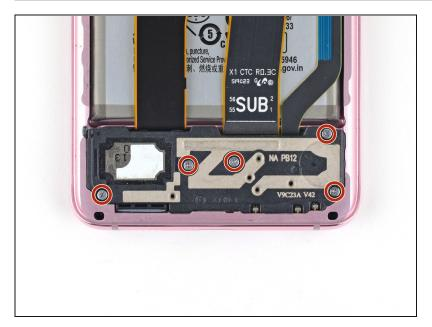
Use a Phillips #00 screwdriver to remove the five 4 mm-long screws securing the loudspeaker and lower midframe.
