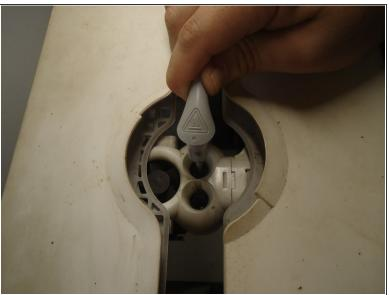
On the top of the printer, turn the injector counter-clockwise and pull the tab.
