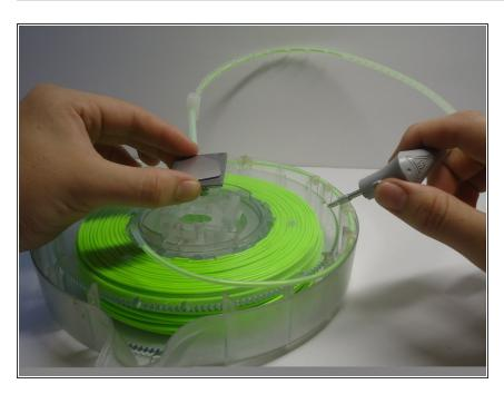
Flip the cartridge face up and remove the gearbox and extractor tube.
