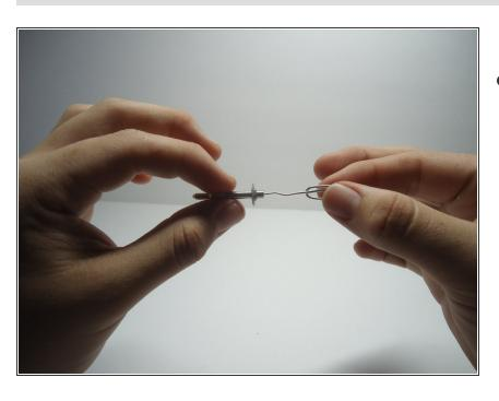
Insert a paper clip and turn until the clog is removed. To reassemble your device, follow these instructions in reverse order.
