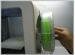
Insert your fingers in the center of the filament cartridge and slowly pull it away from the printer.
