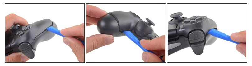
Use the opening tool to separate the panels by releasing the plastic clips around the perimeter of the controller.
