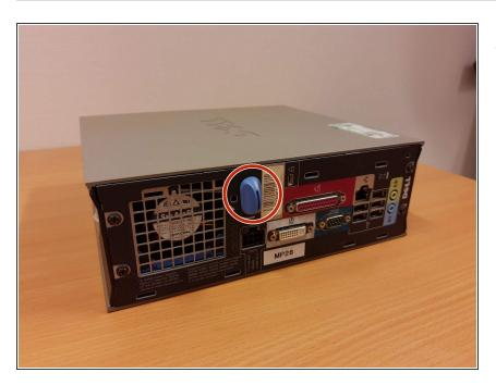
Start by removing the side panel by rotating the blue knob in the direction of the arrow
