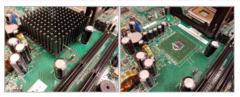
Remove the heat sink for the graphics chip by pressing the metal tab down and out of the hole.
