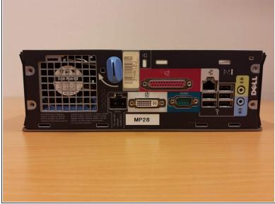
Unscrew the four screws on the back.
