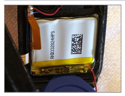
Gently pry the battery out from the side where the electronics sits and the cable is connected. Take your time as the battery is glued in.
