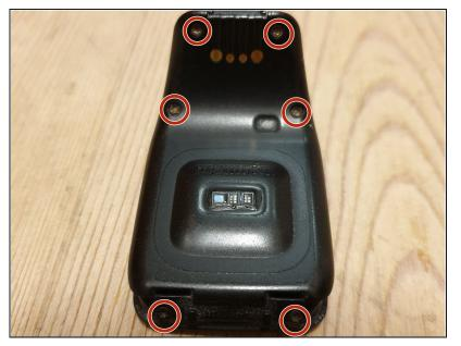
• Unscrew the six Torx 5 Srews with a Srewdriver. Better results are achieved if you memorize the location of the screws, as they are screwed into the plastic housing of the watch.
