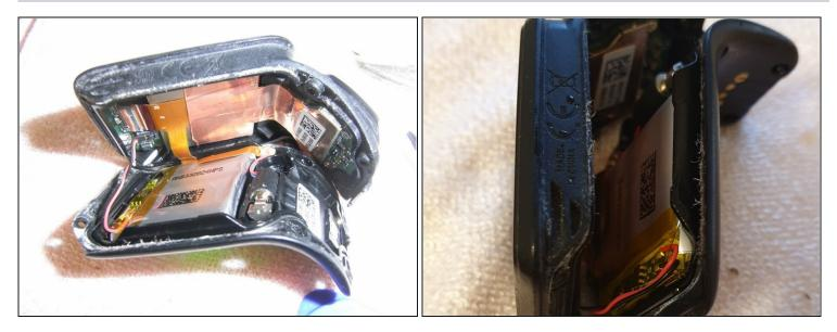
• Gently open the housing, if the two halves do not come apart, gently pry on the halves with the prying tool / plastic card.
