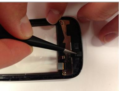
Find the rubber microphone backing on the bottom of the back of the front cover as shown in the picture. Use tweezers to pluck the microphone from the casing.
