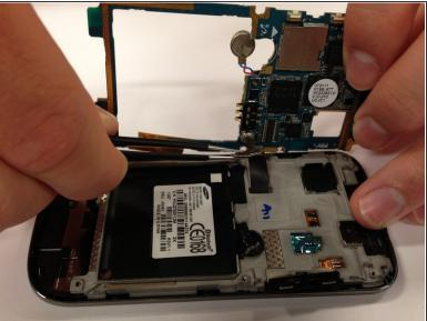
NOT remove the motherboard completely. One more clip on the motherboard's backside needs to be removed.
