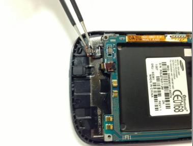
• On the right from the lever, use the tweezers to unclip the black connector.
