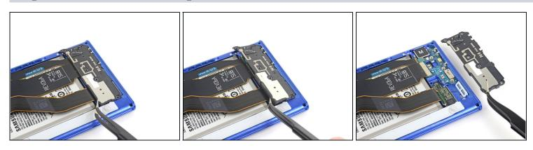
• Use a pair of <u>tweezers</u> to remove the loudspeaker.
