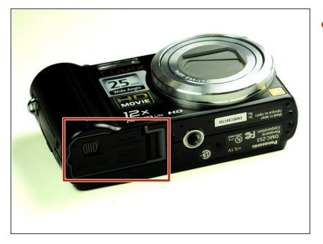
• Locate the small, hinged door on the bottom of the camera.
